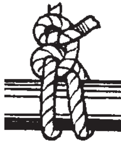
Round Turn and Two Half Hitches
